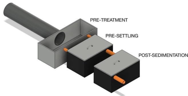
*Figure 5. Isometric view of the SmartSeptic system.*
